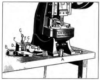
Fig. 10. Tools for Perforating Special Cylindrical Shells
